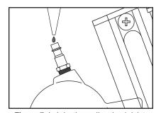
Figure 7. Lubricating nailer via air inlet.
